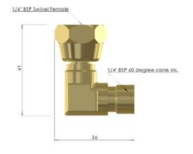
90 degree adaptor connecting the master cylinder valve to the slave/master cylinder valve
